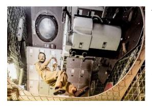
The triangle on the bottom of this mannequin astronaut's shoe fits in the slots on the wall so he doesn't "float" away.
